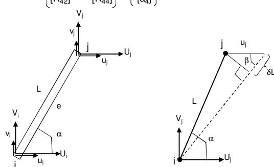
Let us induce a small displacement  $u_j$ , keeping other nodal displacement components equal to zero. The elongation  $\delta L$  of the member is then  $\delta L = u_j \cos\beta$ . For small displacement  $u_j$ , we can take angle  $\alpha \approx \beta$ . Hence,  $\delta L \approx u_j \cos\alpha$ .
